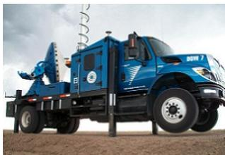
The Flexible Array of Radars and Mesonets (FARM) consists of DOW radars, mobile mesonets, mobile upper air sounding systems, disdrometers, and deployable instrumentation pods used to service the scientific community. The DOW radars have been used in numerous field campaigns including VORTEX2, PECAN, OLYMPEX, SNOWIE, RELAMPAGO, VORTEX-SE, and more! We are really excited to have this facility on campus!
