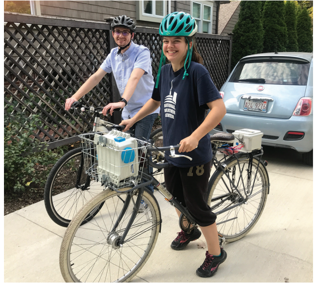
Undergraduate students Marley Majetic and Alex Bruchhauser prepare for a bike ride to measure air quality with ARISense in Urbana-Champaign
